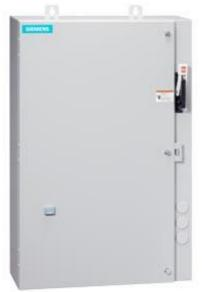
Non-reversing motor starter Size 0 Three phase full voltage Amb compensate bimetal OLrelay Contactor amp rating 18Amp 110V 50HZ / 120V 60HZ coil Combination type 25Amp circuit breaker Encl NEMA type 4X 304 S-steel Water/dust tight noncorrosive Extra-wide enclosure
