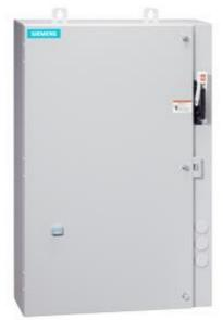
Non-reversing motor starter Size 0 Three phase full voltage Amb compensate bimetal OLrelay Contactor amp rating 18Amp 190-220/220-240V 50/60HZ coil Combination type 25Amp circuit breaker Encl NEMA type 4X 304 S-steel Water/dust tight noncorrosive Extrawide enclosure
