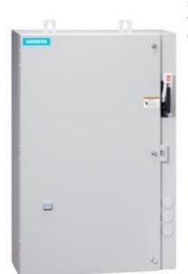
Non-reversing motor starter Size 0 Three phase full voltage Amb compensate bimetal OLrelay Contactor amp rating 18Amp 24VAC 50-60HZ coil Combination type 25Amp circuit breaker Encl NEMA type 4X 304 S-steel Water/dust tight noncorrosive Extra-wide enclosure
