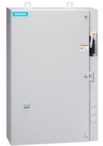
Non-reversing motor starter Size 0 Three phase full voltage Amb compensate bimetal OLrelay Contactor amp rating 18Amp 240V 50HZ / 277V 60HZ coil Combination type 25Amp circuit breaker Encl NEMA type 4X 304 S-steel Water/dust tight noncorrosive Extra-wide enclosure
