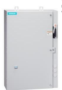
Non-reversing motor starter Size 0 Three phase full voltage Amb compensate bimetal OLrelay Contactor amp rating 18Amp 110-120/220-240VAC 60HZ coil Combination type 3Amp circuit breaker Encl NEMA type 4X 316 S-steel Water/dust tight noncorrosive Extrawide enclosure
