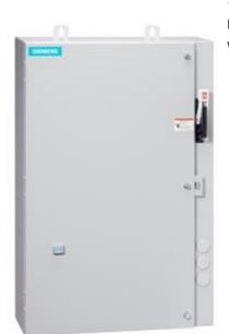
Non-reversing motor starter Size 0 Three phase full voltage Amb compensate bimetal OLrelay Contactor amp rating 18Amp 110-120/220-240VAC 60HZ coil Combination type 3Amp circuit breaker Encl NEMA type 4X 316 S-steel Water/dust tight noncorrosive Extrawide enclosure
