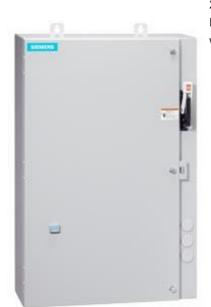
Non-reversing motor starter Size 0 Three phase full voltage Amb compensate bimetal OLrelay Contactor amp rating 18Amp 220-240/440-480VAC 60HZ coil Combination type 3Amp circuit breaker Encl NEMA type 4X 316 S-steel Water/dust tight noncorrosive Extrawide enclosure
