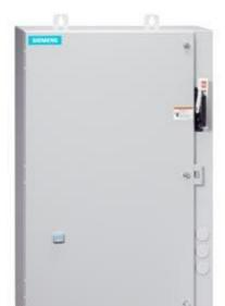
Non-reversing motor starter Size 0 Three phase full voltage Amb compensate bimetal OLrelay Contactor amp rating 18Amp 208VAC 60HZ coil Combination type 3Amp circuit breaker Encl NEMA type 4X 316 S-steel Water/dust tight noncorrosive Extra-wide enclosure
