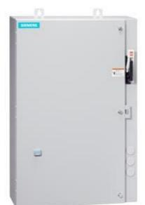
Non-reversing motor starter Size 0 Three phase full voltage Amb compensate bimetal OLrelay Contactor amp rating 18Amp 208VAC 60HZ coil Combination type 3Amp circuit breaker Encl NEMA type 4X 316 S-steel Water/dust tight noncorrosive Extra-wide enclosure
