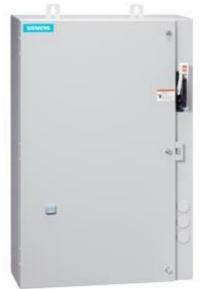
Non-reversing motor starter Size 0 Three phase full voltage Amb compensate bimetal OLrelay Contactor amp rating 18Amp 110V 50HZ / 120V 60HZ coil Combination type 3Amp circuit breaker Encl NEMA type 4X 316 S-steel Water/dust tight noncorrosive Extra-wide enclosure
