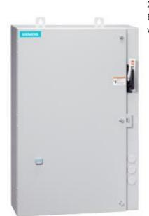
Non-reversing motor starter Size 0 Three phase full voltage Amb compensate bimetal OLrelay Contactor amp rating 18Amp 190-220/220-240V 50/60HZ coil Combination type 3Amp circuit breaker Encl NEMA type 4X 316 S-steel Water/dust tight noncorrosive Extrawide enclosure
