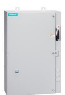
Non-reversing motor starter Size 0 Three phase full voltage Amb compensate bimetal OLrelay Contactor amp rating 18Amp 24VAC 50-60HZ coil Combination type 3Amp circuit breaker Encl NEMA type 4X 316 S-steel Water/dust tight noncorrosive Extra-wide enclosure
