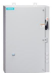
Non-reversing motor starter Size 0 Three phase full voltage Amb compensate bimetal OLrelay Contactor amp rating 18Amp 208VAC 60HZ coil Combination type 10Amp circuit breaker Encl NEMA type 4X 316 S-steel Water/dust tight noncorrosive Extra-wide enclosure
