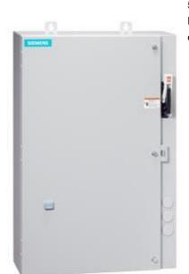
Non-reversing motor starter Size 0 Three phase full voltage Amb compensate bimetal OLrelay Contactor amp rating 18Amp 110V 50HZ / 120V 60HZ coil Combination type 10Amp circuit breaker Encl NEMA type 4X 316 S-steel Water/dust tight noncorrosive Extra-wide enclosure
