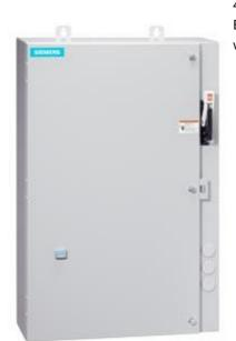
Non-reversing motor starter Size 0 Three phase full voltage Amb compensate bimetal OLrelay Contactor amp rating 18Amp 380-440/440-480V 50/60HZ coil Combination type 10Amp circuit breaker Encl NEMA type 4X 316 S-steel Water/dust tight noncorrosive Extrawide enclosure
