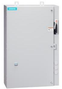
Non-reversing motor starter Size 0 Three phase full voltage Amb compensate bimetal OLrelay Contactor amp rating 18Amp 240V 50HZ / 277V 60HZ coil Combination type 10Amp circuit breaker Encl NEMA type 4X 316 S-steel Water/dust tight noncorrosive Extra-wide enclosure
