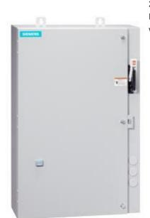
Non-reversing motor starter Size 0 Three phase full voltage Amb compensate bimetal OLrelay Contactor amp rating 18Amp 220-240/440-480VAC 60HZ coil Combination type 25Amp circuit breaker Encl NEMA type 4X 316 S-steel Water/dust tight noncorrosive Extrawide enclosure
