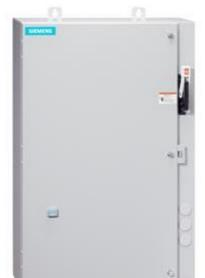
Non-reversing motor starter Size 0 Three phase full voltage Amb compensate bimetal OLrelay Contactor amp rating 18Amp 208VAC 60HZ coil Combination type 25Amp circuit breaker Encl NEMA type 4X 316 S-steel Water/dust tight noncorrosive Extra-wide enclosure
