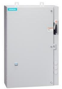
Non-reversing motor starter Size 0 Three phase full voltage Amb compensate bimetal OLrelay Contactor amp rating 18Amp 190-220/220-240V 50/60HZ coil Combination type 25Amp circuit breaker Encl NEMA type 4X 316 S-steel Water/dust tight noncorrosive Extrawide enclosure
