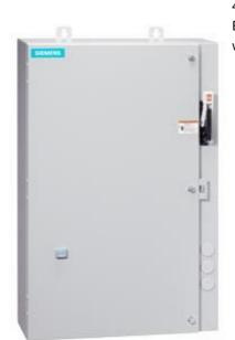
Non-reversing motor starter Size 0 Three phase full voltage Amb compensate bimetal OLrelay Contactor amp rating 18Amp 380-440/440-480V 50/60HZ coil Combination type 25Amp circuit breaker Encl NEMA type 4X 316 S-steel Water/dust tight noncorrosive Extrawide enclosure
