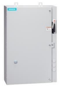
Non-reversing motor starter Size 0 Three phase full voltage Amb compensate bimetal OLrelay Contactor amp rating 18Amp 24VAC 50-60HZ coil Combination type 25Amp circuit breaker Encl NEMA type 4X 316 S-steel Water/dust tight noncorrosive Extra-wide enclosure
