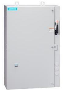
Non-reversing motor starter Size 0 Three phase full voltage Amb compensate bimetal OLrelay Contactor amp rating 18Amp 240V 50HZ / 277V 60HZ coil Combination type 25Amp circuit breaker Encl NEMA type 4X 316 S-steel Water/dust tight noncorrosive Extra-wide enclosure
