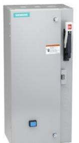
Non-reversing motor starter Size 0 Three phase full voltage Amb compensate bimetal OLrelay Contactor amp rating 18Amp 24VAC 50-60HZ coil Combination type 10Amp circuit breaker Enclosure NEMA type 1 Indoor general purpose use Standard width enclosure
