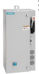
Non-reversing motor starter Size 0 Three phase full voltage Amb compensate bimetal OLrelay Contactor amp rating 18Amp 550/575-600 50/60HZ coil Combination type 3Amp circuit breaker Enclosure NEMA type 4/12 Water/dust tight for outdoors Standard width enclosure
