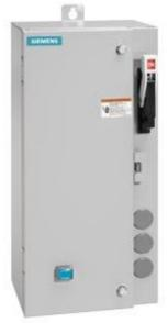
Non-reversing motor starter Size 0 Three phase full voltage Amb compensate bimetal OLrelay Contactor amp rating 18Amp 110V 50HZ / 120V 60HZ coil Combination type 3Amp circuit breaker Enclosure NEMA type 4/12 Water/dust tight for outdoors Standard width enclosure
