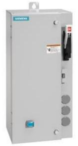
Non-reversing motor starter Size 0 Three phase full voltage Amb compensate bimetal OLrelay Contactor amp rating 18Amp 110V 50HZ / 120V 60HZ coil Combination type 3Amp circuit breaker Enclosure NEMA type 4/12 Water/dust tight for outdoors Standard width enclosure
