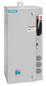
Non-reversing motor starter Size 0 Three phase full voltage Amb compensate bimetal OLrelay Contactor amp rating 18Amp 380-440/440-480V 50/60HZ coil Combination type 3Amp circuit breaker Enclosure NEMA type 4/12 Water/dust tight for outdoors Standard width enclosure
