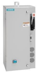
Non-reversing motor starter Size 0 Three phase full voltage Amb compensate bimetal OLrelay Contactor amp rating 18Amp 24VAC 50-60HZ coil Combination type 3Amp circuit breaker Enclosure NEMA type 4/12 Water/dust tight for outdoors Standard width enclosure
