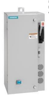
Non-reversing motor starter Size 0 Three phase full voltage Amb compensate bimetal OLrelay Contactor amp rating 18Amp 240V 50HZ / 277V 60HZ coil Combination type 3Amp circuit breaker Enclosure NEMA type 4/12 Water/dust tight for outdoors Standard width enclosure
