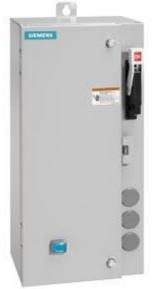
Non-reversing motor starter Size 0 Three phase full voltage Amb compensate bimetal OLrelay Contactor amp rating 18Amp 110-120/220-240VAC 60HZ coil Combination type 10Amp circuit breaker Enclosure NEMA type 4/12 Water/dust tight for outdoors Standard width enclosure
