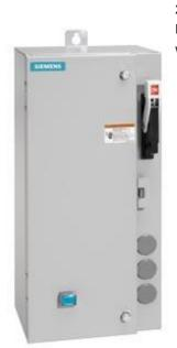
Non-reversing motor starter Size 0 Three phase full voltage Amb compensate bimetal OLrelay Contactor amp rating 18Amp 220-240/440-480VAC 60HZ coil Combination type 10Amp circuit breaker Enclosure NEMA type 4/12 Water/dust tight for outdoors Standard width enclosure
