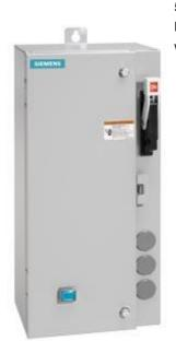
Non-reversing motor starter Size 0 Three phase full voltage Amb compensate bimetal OLrelay Contactor amp rating 18Amp 110V 50HZ / 120V 60HZ coil Combination type 10Amp circuit breaker Enclosure NEMA type 4/12 Water/dust tight for outdoors Standard width enclosure
