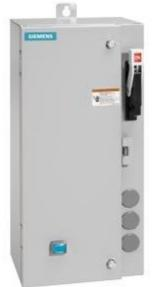
Non-reversing motor starter Size 0 Three phase full voltage Amb compensate bimetal OLrelay Contactor amp rating 18Amp 190-220/220-240V 50/60HZ coil Combination type 10Amp circuit breaker Enclosure NEMA type 4/12 Water/dust tight for outdoors Standard width enclosure
