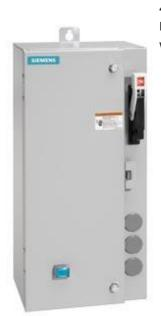
Non-reversing motor starter Size 0 Three phase full voltage Amb compensate bimetal OLrelay Contactor amp rating 18Amp 380-440/440-480V 50/60HZ coil Combination type 10Amp circuit breaker Enclosure NEMA type 4/12 Water/dust tight for outdoors Standard width enclosure
