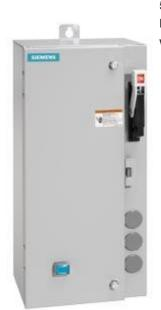
Non-reversing motor starter Size 0 Three phase full voltage Amb compensate bimetal OLrelay Contactor amp rating 18Amp 240V 50HZ / 277V 60HZ coil Combination type 10Amp circuit breaker Enclosure NEMA type 4/12 Water/dust tight for outdoors Standard width enclosure
