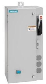
Non-reversing motor starter Size 0 Three phase full voltage Amb compensate bimetal OLrelay Contactor amp rating 18Amp 110-120/220-240VAC 60HZ coil Combination type 25Amp circuit breaker Enclosure NEMA type 4/12 Water/dust tight for outdoors Standard width enclosure
