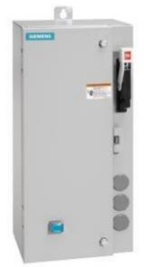
Non-reversing motor starter Size 0 Three phase full voltage Amb compensate bimetal OLrelay Contactor amp rating 18Amp 220-240/440-480VAC 60HZ coil Combination type 25Amp circuit breaker Enclosure NEMA type 4/12 Water/dust tight for outdoors Standard width enclosure
