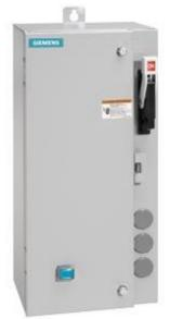
Non-reversing motor starter Size 0 Three phase full voltage Amb compensate bimetal OLrelay Contactor amp rating 18Amp 550/575-600 50/60HZ coil Combination type 25Amp circuit breaker Enclosure NEMA type 4/12 Water/dust tight for outdoors Standard width enclosure
