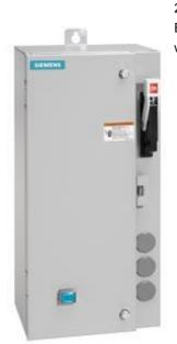
Non-reversing motor starter Size 0 Three phase full voltage Amb compensate bimetal OLrelay Contactor amp rating 18Amp 190-220/220-240V 50/60HZ coil Combination type 25Amp circuit breaker Enclosure NEMA type 4/12 Water/dust tight for outdoors Standard width enclosure
