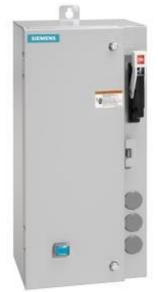
Non-reversing motor starter Size 0 Three phase full voltage Amb compensate bimetal OLrelay Contactor amp rating 18Amp 380-440/440-480V 50/60HZ coil Combination type 25Amp circuit breaker Enclosure NEMA type 4/12 Water/dust tight for outdoors Standard width enclosure
