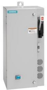
Non-reversing motor starter Size 0 Three phase full voltage Amb compensate bimetal OLrelay Contactor amp rating 18Amp 240V 50HZ / 277V 60HZ coil Combination type 25Amp circuit breaker Enclosure NEMA type 4/12 Water/dust tight for outdoors Standard width enclosure
