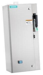
Non-reversing motor starter Size 0 Three phase full voltage Amb compensate bimetal OLrelay Contactor amp rating 18Amp 110-120/220-240VAC 60HZ coil Combination type 3Amp circuit breaker Encl NEMA type 4X 304 S-steel Water/dust tight noncorrosive Standard width enclosure
