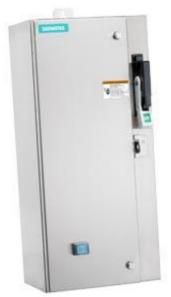
Non-reversing motor starter Size 0 Three phase full voltage Amb compensate bimetal OLrelay Contactor amp rating 18Amp 208VAC 60HZ coil Combination type 3Amp circuit breaker Encl NEMA type 4X 304 S-steel Water/dust tight noncorrosive Standard width enclosure
