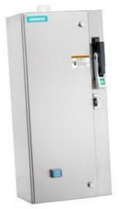
Non-reversing motor starter Size 0 Three phase full voltage Amb compensate bimetal OLrelay Contactor amp rating 18Amp 110V 50HZ / 120V 60HZ coil Combination type 3Amp circuit breaker Encl NEMA type 4X 304 S-steel Water/dust tight noncorrosive Standard width enclosure
