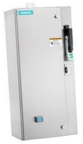
Non-reversing motor starter Size 0 Three phase full voltage Amb compensate bimetal OLrelay Contactor amp rating 18Amp 380-440/440-480V 50/60HZ coil Combination type 3Amp circuit breaker Encl NEMA type 4X 304 S-steel Water/dust tight noncorrosive Standard width enclosure
