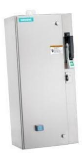
Non-reversing motor starter Size 0 Three phase full voltage Amb compensate bimetal OLrelay Contactor amp rating 18Amp 24VAC 50-60HZ coil Combination type 3Amp circuit breaker Encl NEMA type 4X 304 S-steel Water/dust tight noncorrosive Standard width enclosure
