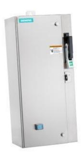
Non-reversing motor starter Size 0 Three phase full voltage Amb compensate bimetal OLrelay Contactor amp rating 18Amp 240V 50HZ / 277V 60HZ coil Combination type 3Amp circuit breaker Encl NEMA type 4X 304 S-steel Water/dust tight noncorrosive Standard width enclosure
