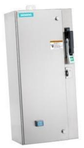
Non-reversing motor starter Size 0 Three phase full voltage Amb compensate bimetal OLrelay Contactor amp rating 18Amp 220-240/440-480VAC 60HZ coil Combination type 10Amp circuit breaker Encl NEMA type 4X 304 S-steel Water/dust tight noncorrosive Standard width enclosure
