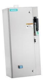
Non-reversing motor starter Size 0 Three phase full voltage Amb compensate bimetal OLrelay Contactor amp rating 18Amp 208VAC 60HZ coil Combination type 10Amp circuit breaker Encl NEMA type 4X 304 S-steel Water/dust tight noncorrosive Standard width enclosure
