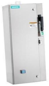
Non-reversing motor starter Size 0 Three phase full voltage Amb compensate bimetal OLrelay Contactor amp rating 18Amp 110V 50HZ / 120V 60HZ coil Combination type 10Amp circuit breaker Encl NEMA type 4X 304 S-steel Water/dust tight noncorrosive Standard width enclosure
